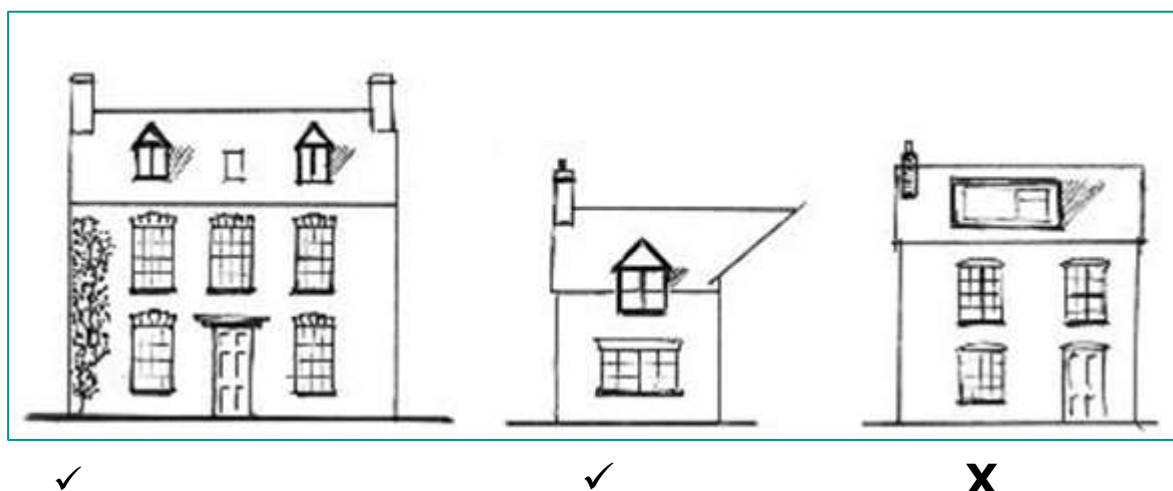
Fig. E20 – good and poor examples of dormer windows.
