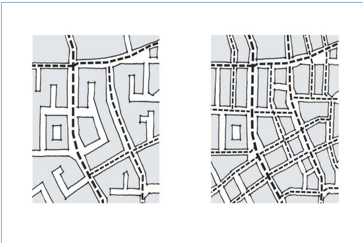
Fig. C.1 - Poor connectivity and good connectivity.
