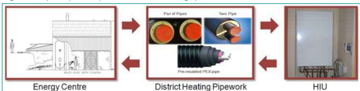
Fig. Q2 - Key component parts of district heating systems.
