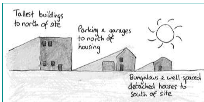
Fig. D7 – Over shading by other buildings should be minimised.
